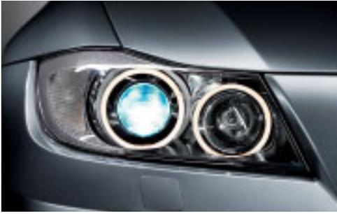
□ **Xenon headlights for low and high beam, including four parking light rings** and automatic headlight range control, provide much better illumination of the road ahead at night or in poor visibility.
