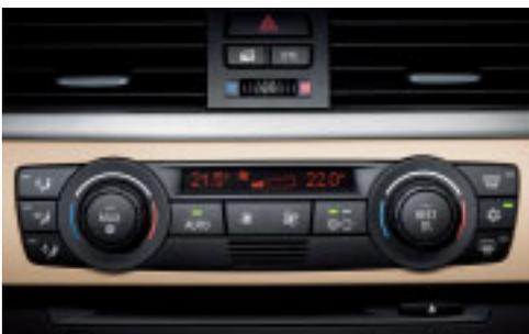
□ **Automatic air conditioning**, incl. AAR, micro filter, fogging and solar sensors and residual heat button, rapidly provides the desired climatic conditions in the vehicle interior and maintains the selected temperature. With individual temperature control at the front (left/right) and climatized storage compartment in the centre console, incl. rear air vent and air conditioning.
