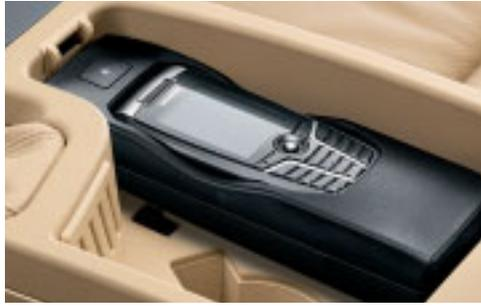
□ **Preparation for mobile phone with Bluetooth interface**, including hands-free facility, connection for charger and outside aerial. A separately available snap-in adapter enables connection of a Bluetooth-compatible mobile phone, which can also be operated via the iDrive Controller (in conjunction with navigation system). For mobile phone options contact your BMW partner.
