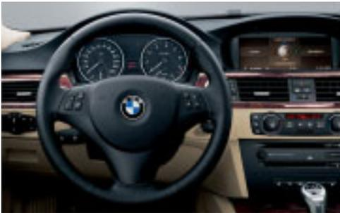
□ **Leather sports steering wheel** (369 mm diameter), three spokes, incl. gearshift lever handle with chrome trim and handbrake lever handle finished in leather, multifunction buttons for remote control of radio/telephone (both optional); also available without multifunction buttons.
