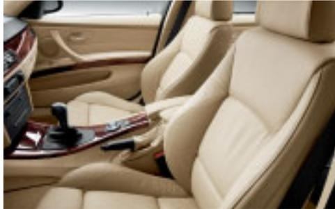
□ **Sports seats** for driver and front passenger (shown here in optionally available Dakota leather Beige). Optimum lateral support is ensured by continuously variable electric backrest width adjustment. Seat height, backrest and seat angle as well as thigh support are manually adjustable.
