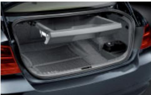
□ **Luggage compartment package** including luggage compartment floor net, 12 V socket, segmentable underfloor storage bin, bag and umbrella holder, waterproof folding box and a pull-out drawer under the rear shelf. If the drawer is not required, it is quick and easy to remove.
