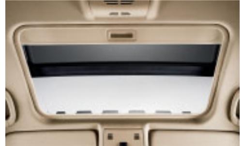
□ **Glass sliding/vent roof**, electric, with wind deflector and comfort opening function via the car's remote control unit, includes reading lights at the front and illuminated vanity mirrors.
