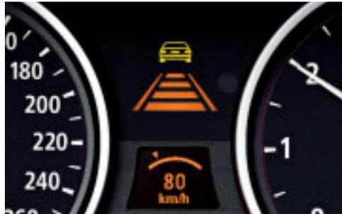
□ **Active Cruise Control** enables comfortable driving at a pre-selected speed. When driving in columns of traffic, your BMW automatically adapts to the speed of the preceding vehicle and uses its radar sensor to maintain a preset distance. In addition, the braking function ensures that the desired speed is maintained even when driving downhill. (Only available for 325i, 330i and 330d.)
